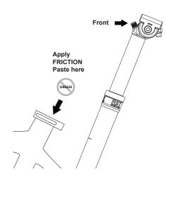
Close the clamp and reinstall screw.
